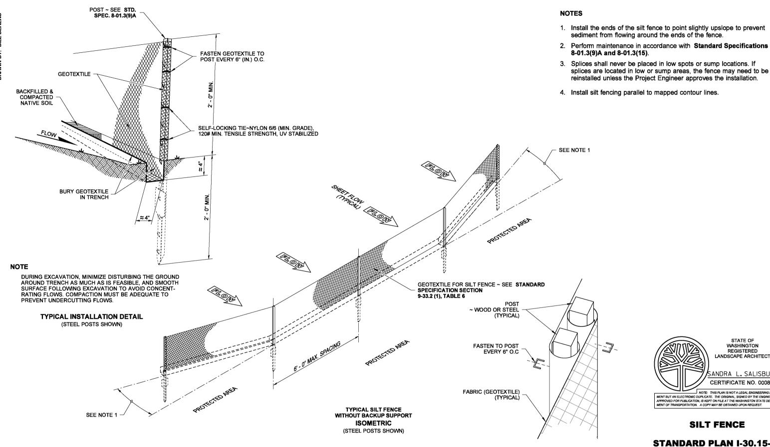
SPLICED FENCE SECTIONS SHALL BE CLOSE ENOUGH TOGETHER TO PREVENT SILT LADEN WATER FROM ESCAPING THROUGH THE FENCE AT THE OVERLAP.
