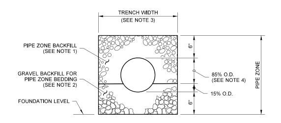
**CONCRETE AND DUCTILE IRON PIPE**
