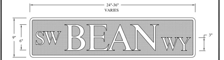
STREET NAME SIGNS SHALL CONSIST OF MIN. 24" TO MAX. 36" BULB EXTRUDED BLANK THE SIZE OF STREET NAMING SIGN WILL DEPEND ON THE LENGTH OF THE STREET NAME.
